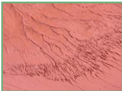
Figure 42: Red mud without hazardous characteristics pH value < 11.5
