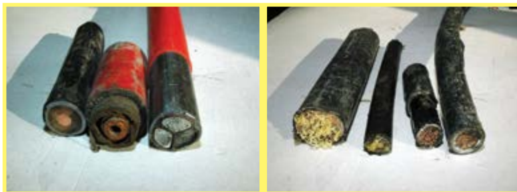
Figure 253: Underground cable (oil insulation)
