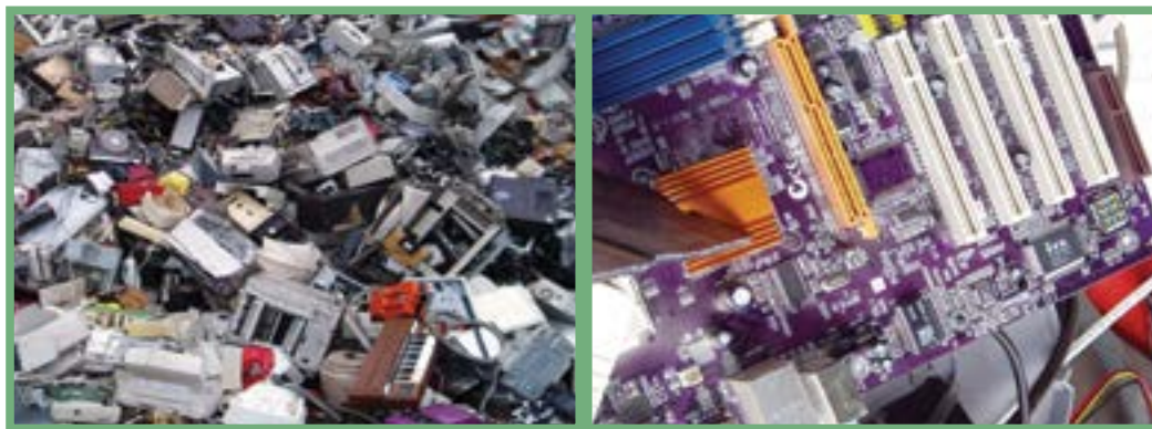
Figure 87: Mixed electronic scrap without devices with environmentally relevant quantities of hazardous components
