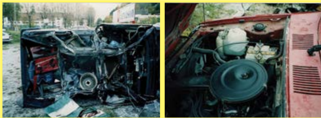
Figure 113: Wrecked car without the hazardous substances removed – unlisted waste
