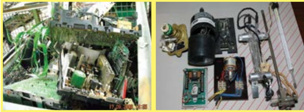
Figure 105: Circuit boards populated with hazardous components – A1180
