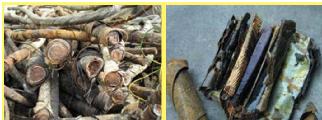
Figure 152: Cable waste with hazardous components – A1190
