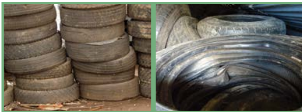
Figure 17: End-of-life tyres without the required tread depth
