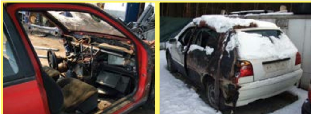
Figure 119: Partially cannibalised wrecked car – unlisted waste
