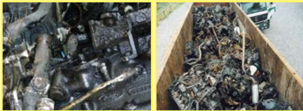
Figure 85: Vehicle engines which have not been emptied of remnants; no verification of functionality – A1180 Figure 86: Vehicle engines which have not been emptied of remnants – A1180
