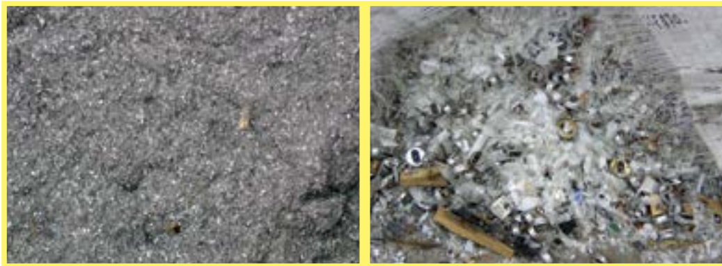
Figure 31: Fine aluminium shavings (20% of the fraction is below 100 \mu\text{m} ) – unlisted waste
