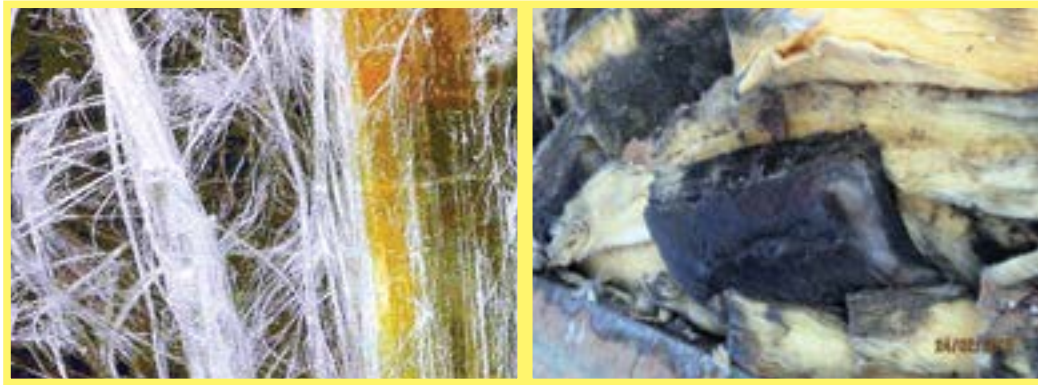
Figure 133: Asbestos fibre – A2050
