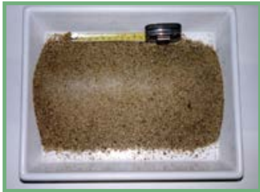
Figure 65: Slag sand (granulated iron slag) – PRODUCT
