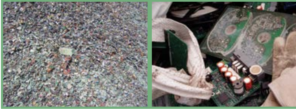
Figure 89: Shredded printed circuit boards previously freed of hazardous components
