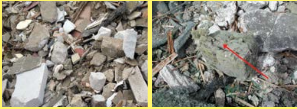
Figure 48: Mixed building waste – unlisted waste
