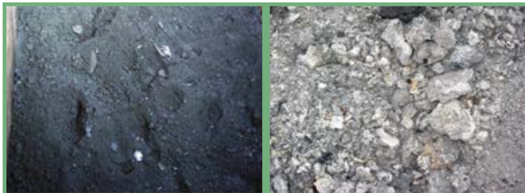
Figure 21: Aluminium skimmings (hazardous characteristic H4.3) – unlisted waste
