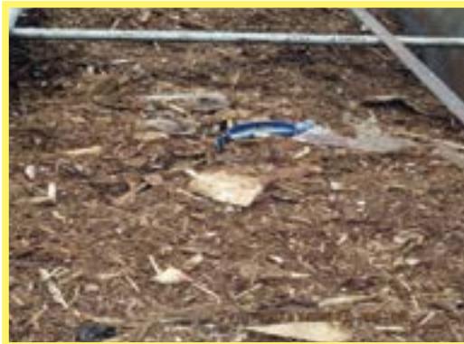
Figure 146: Waste wood with high content of treated waste wood, fine particles and contaminants – AC170
