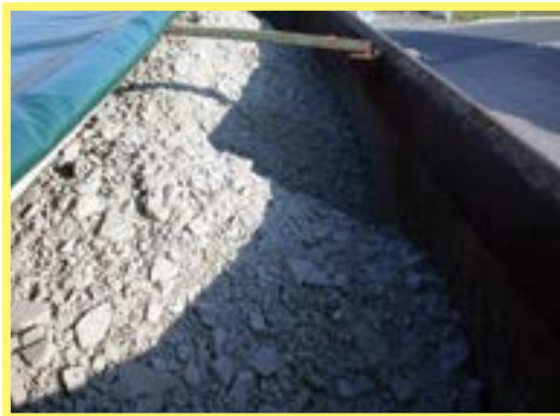
Figure 240: Zinc hydroxide or jarosite sludge (dried) – A1070
