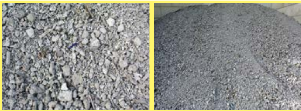
Figure 213: Metal concentrate, mainly aluminium, from incineration slags, a metal percentage under 90% - unlisted waste
