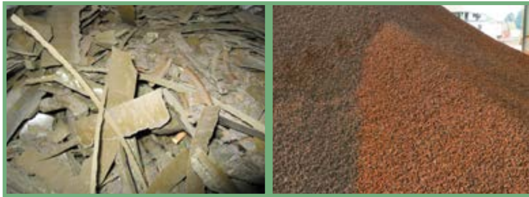
Figure 161: Ceramic waste from the production of ceramic grinding discs
