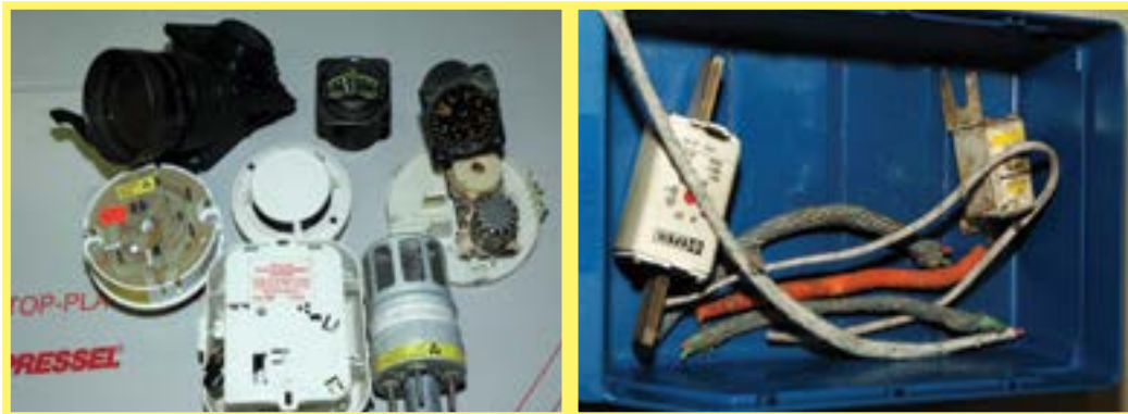
Figure 107: Radioactive components (radiation protection provisions may apply) – A1180
