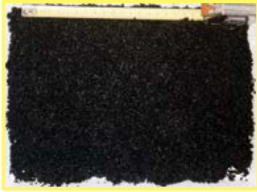
Figure 16: Contaminated activated carbon from water purification – A4160
