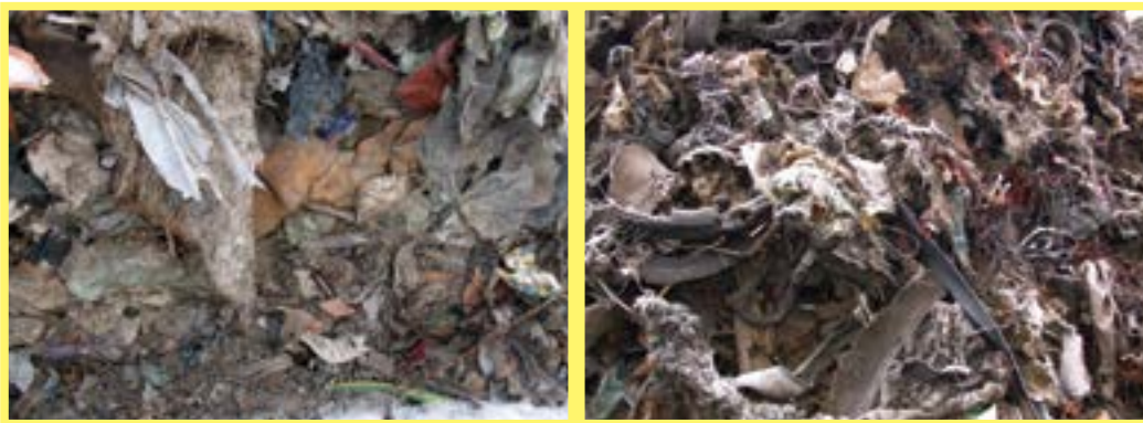
Figure 211: Light shredder fraction – A3120
