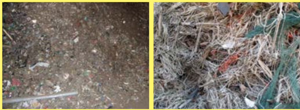
Figure 76: Iron/steel scrap with high impurity content from mechanical-biological treatment plants (MBT) – unlisted waste
