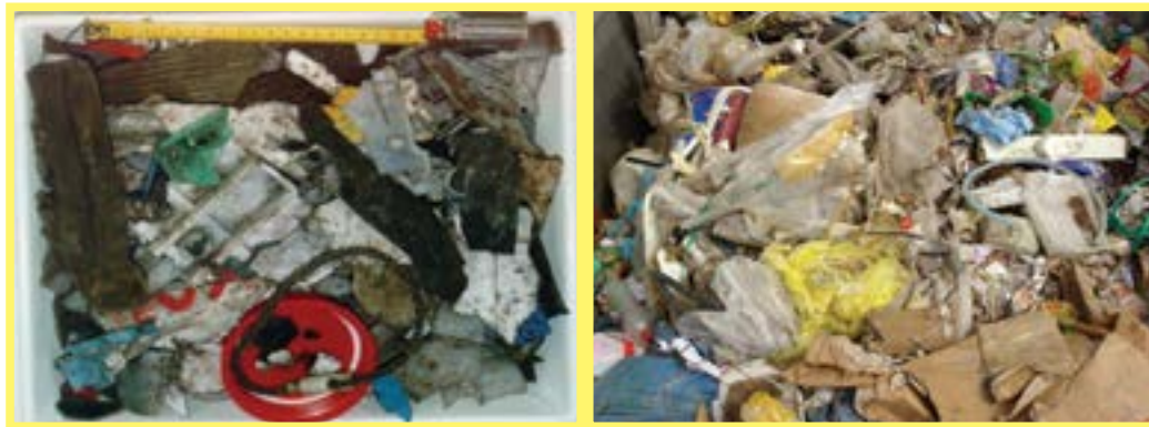
Figure 174: Contaminated polypropylene battery waste – A1020 or A1160
