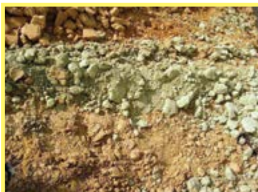
Figure 123: Impure gypsum whose recovery is not ensured – AB150
