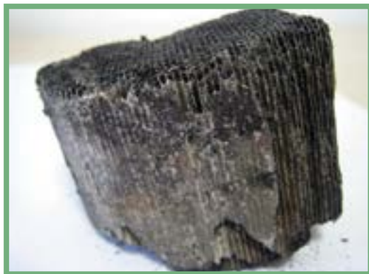
Figure 156: Ceramic monoliths from the dismantling of end-of-life vehicles – Amber List in certain EU Member States
