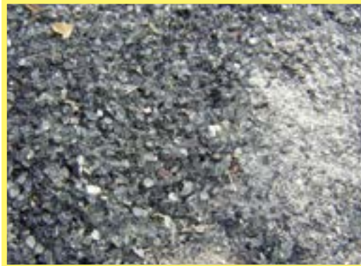
Figure 131: Cleaned cathode ray tube waste (containing lead) – A1020 or A2010
