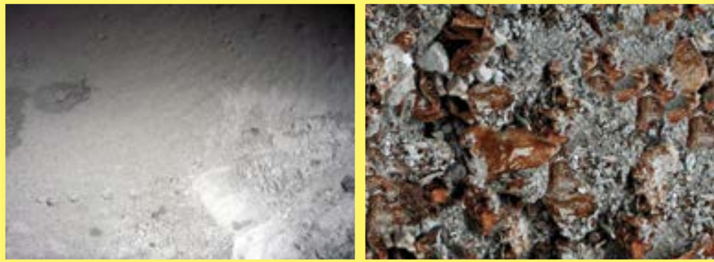
Figure 74: Filter dust from stainless steel casting – A4100
