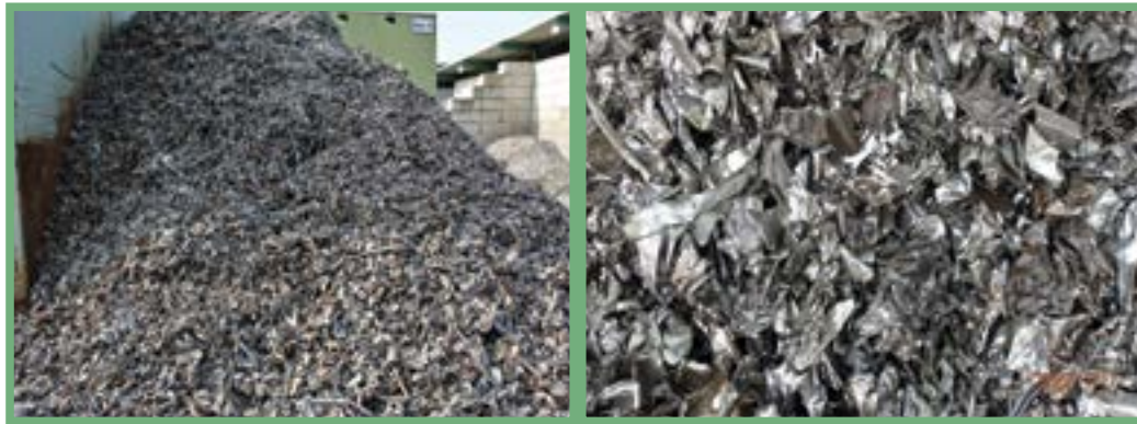
Figure 70: VA stainless steel waste > 90% metal content
