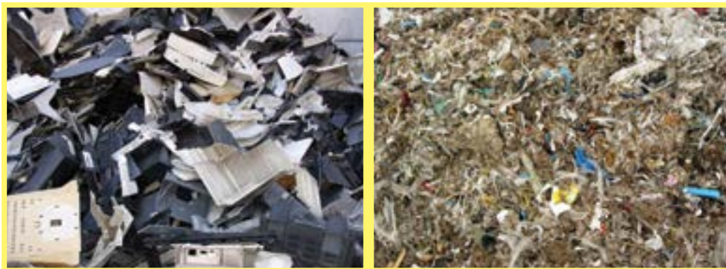
Figure 176: Plastics from monitor rear panels with more than 0.2% bromine content; POP limit values having been exceeded – unlisted waste
