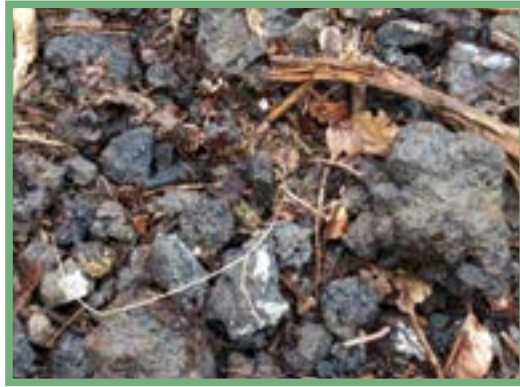
Figure 64: Electrical furnace slag (containing chromium) from a stainless steel mill – Green List in permissible application – NB: Backfilling on soil/roads is illegal!
