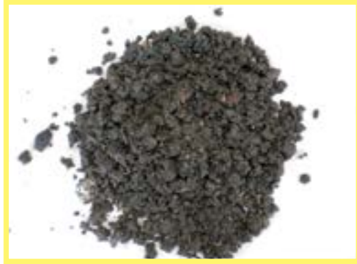
Figure 58: Slag from the combustion of hazardous waste – unlisted waste
