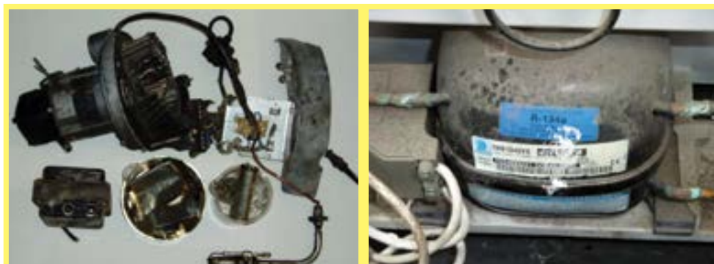
Figure 83: Electric motor with PCB start-up capacitor – A1180
