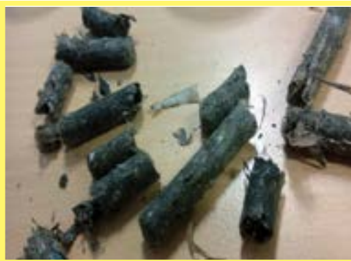
Figure 146: Waste wood with high content of treated waste wood, fine particles and contaminants – AC170
