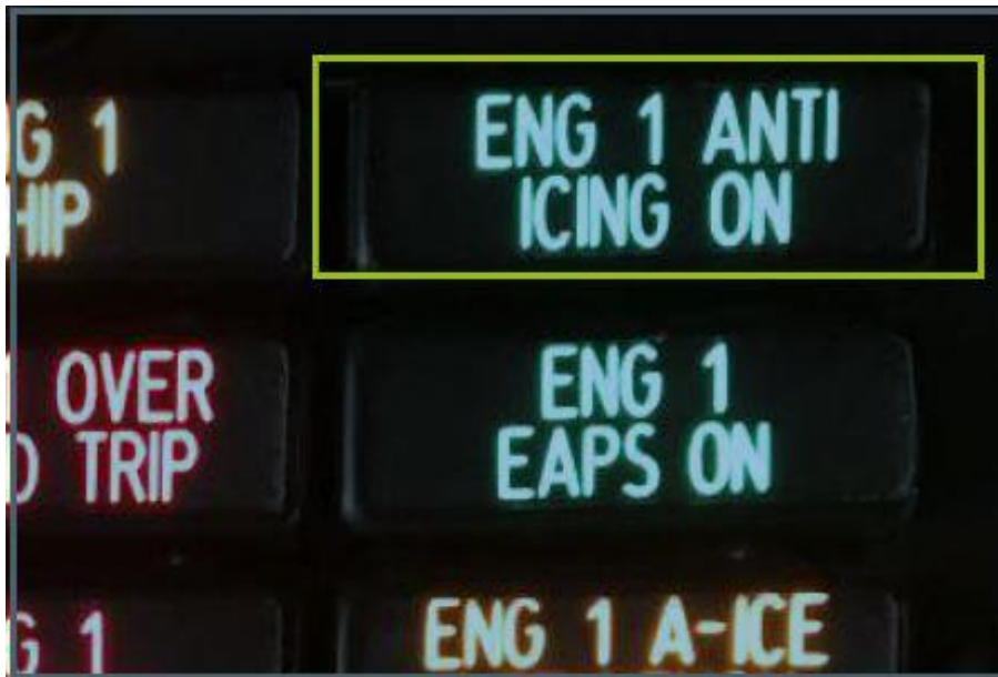
Figure 26: Operation light ENG 1 Anti-Icing ON
