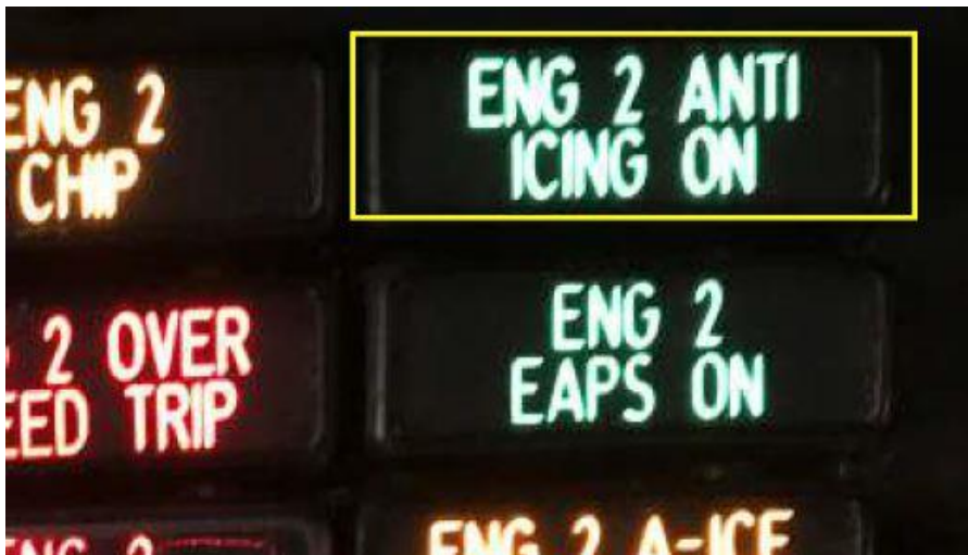
Figure 27: Operation light ENG 2 Anti-Icing ON
