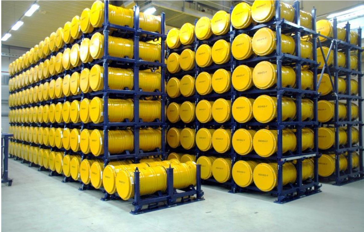
Figure 5 Conditioned waste in interim storage facility 13, © NES
