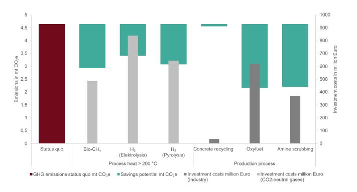
Fuel switch in process heat > 200° C triggers highest investment costs in the sector – provided the costs for the production of CO<sub>2</sub>-neutral gases arise in the industrial sector.
