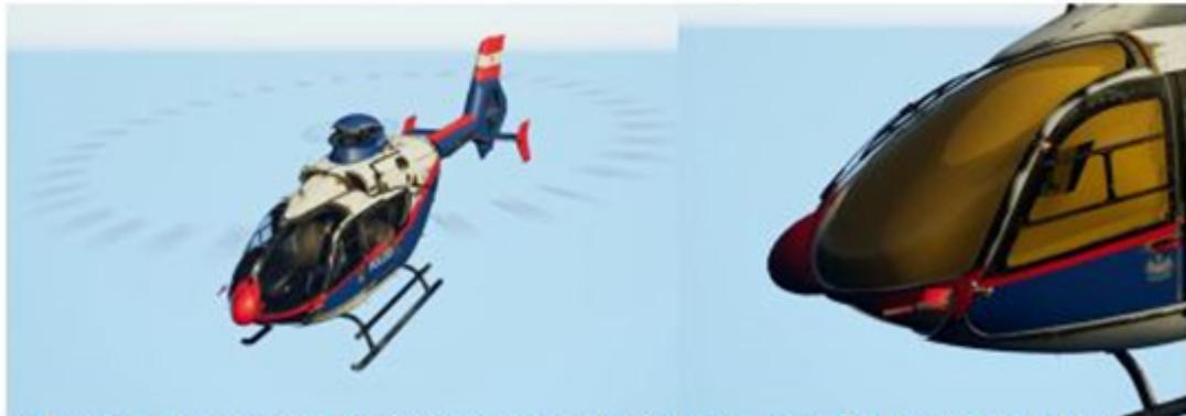
Figure 1: 3D Helicopter Model of EC135P2+ with verified Window Section based on CAD data in yellow (right image)
