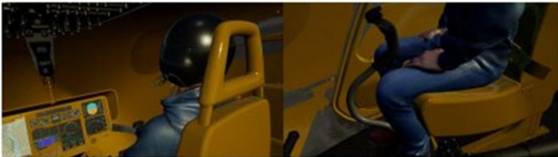
Figure 2: EC135 CAD data overlay (yellow) with 3D Model to verify pilots sitting position and eyepoint
