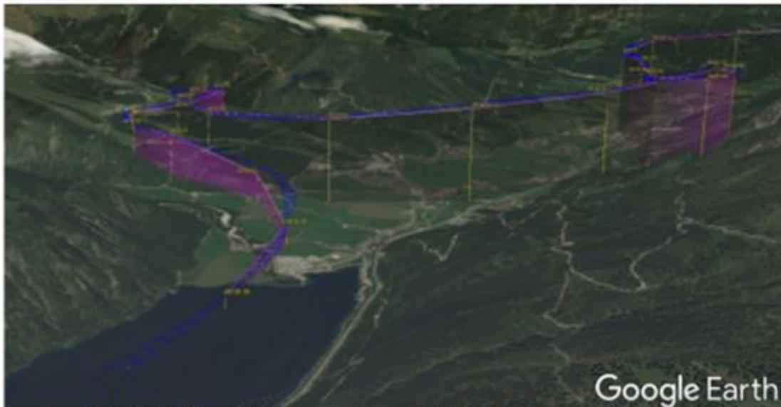
Figure 18: EURONAV Data with timestamps and interpolated flight data & error tunnel (blue), (Google Earth)
