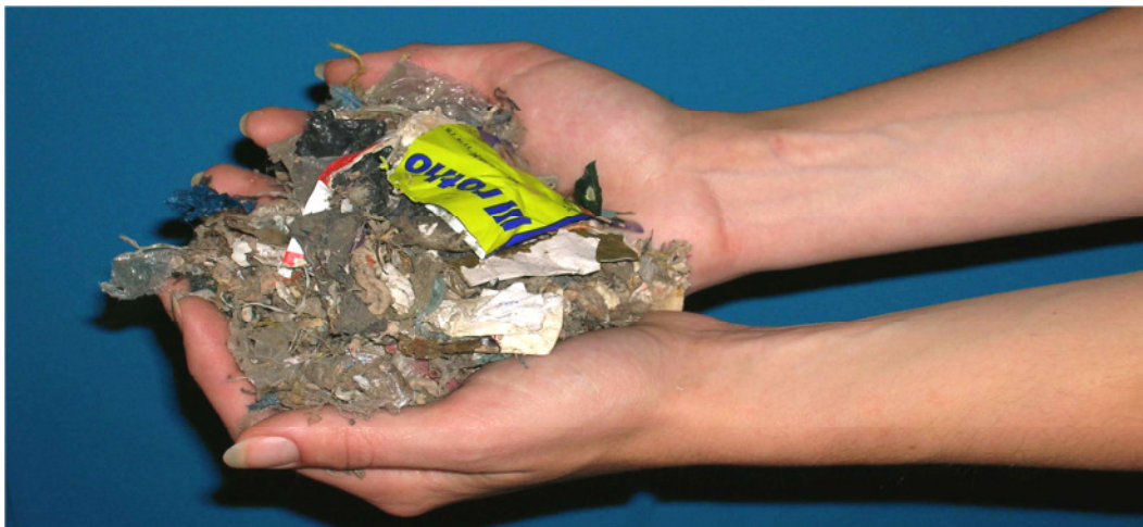
Example of pre-treated waste fuel instead of heating oil as support fuel in the sewage sludge incinerator (input material for fluidized boiler WSO3 in the waste incineration plant Simmering in Vienna)
