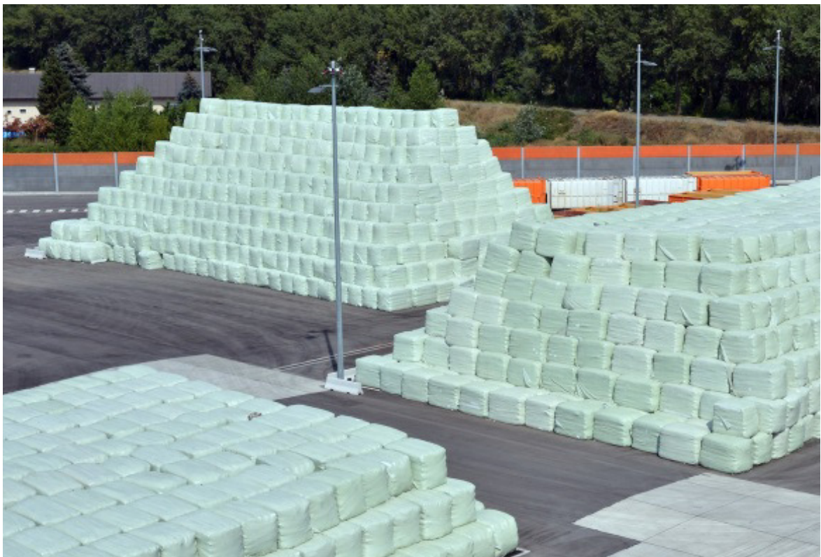
Example for intermediate storage of mechanically processed MSW in Vienna in order to manage seasonal variations in waste generation and temporary shutdown of an incinerator
