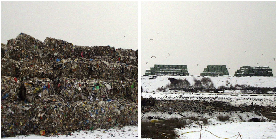
Comparison of alternative intermediate storage at the same point in time at the disposal site Rautenweg, Vienna: The plastic wrapping suppresses heat development – thus layers of snow are only on the plastic wrapped waste (Dez. 2002)
