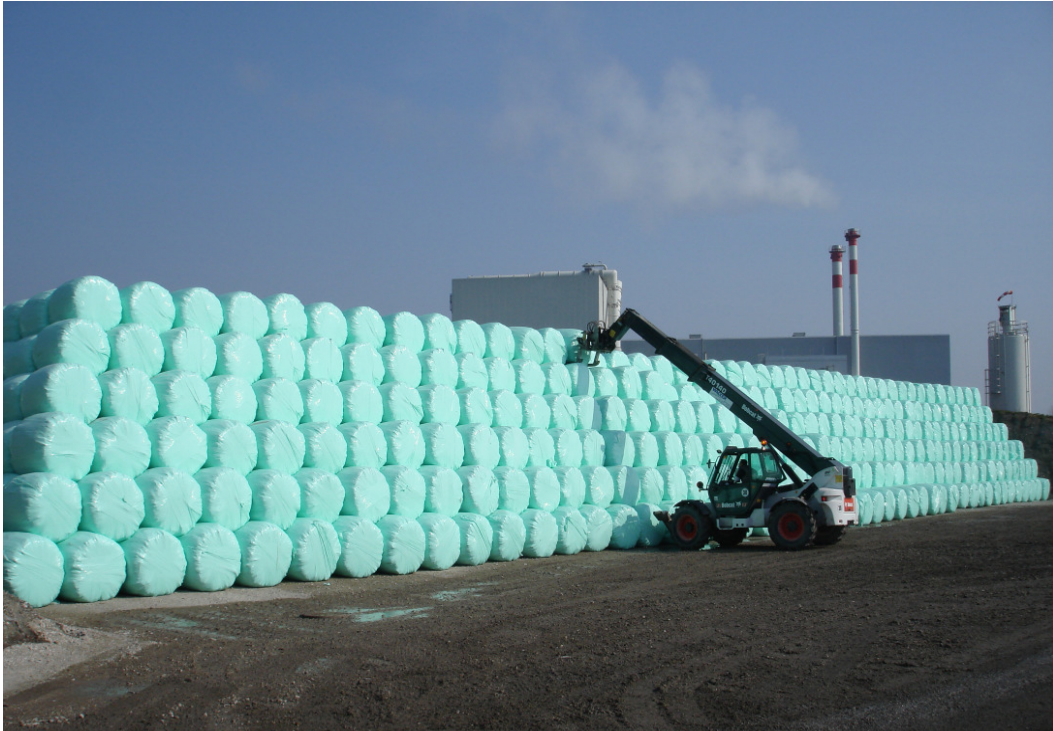
Example of state of the art temporary storage of waste in plastic wrapped bales in Wels (1 bale equals to 2 or 3 barrels of crude oil)
