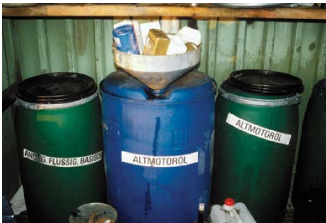
Figure 46: Collection of waste oils
