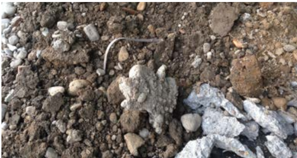
Figure 142: Contaminated excavated material
