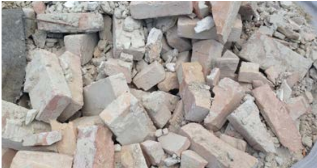
Figure 108: Mineral construction waste generated in the course of the demolition of a building
