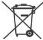
Figure 111: Pictogram of crossed-out waste bin for safeguarding separate collection (Source: Batteries Ordinance)
