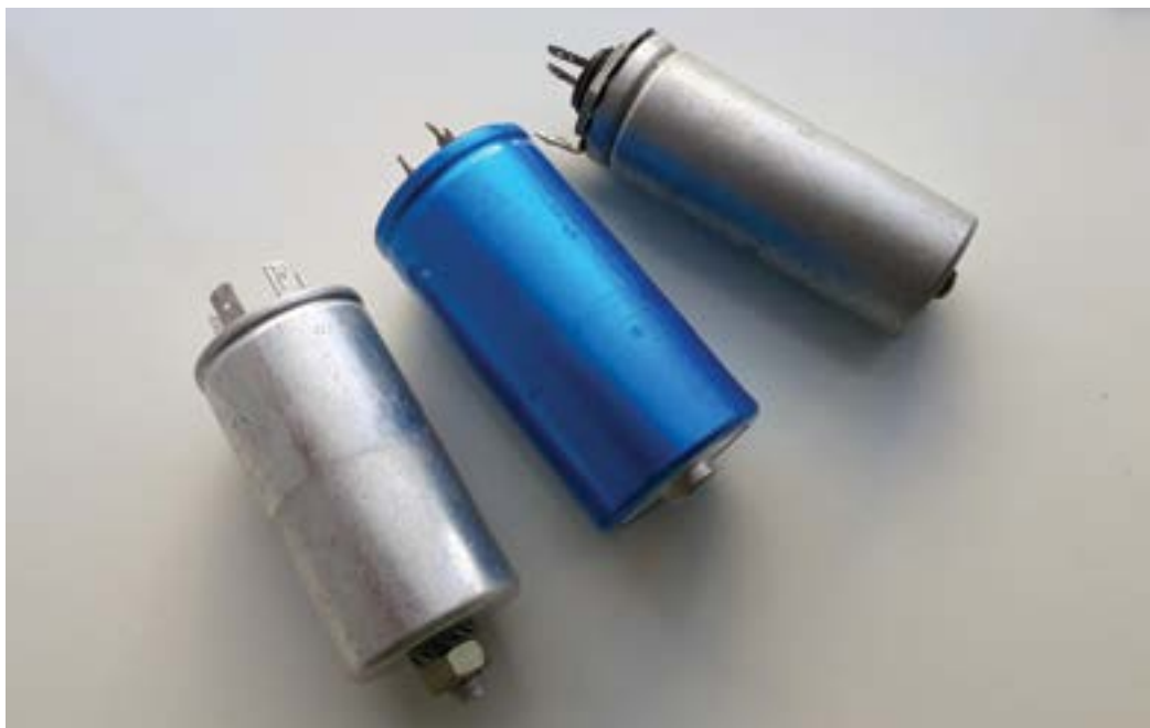
Figure 136: Capacitors containing PCBs
