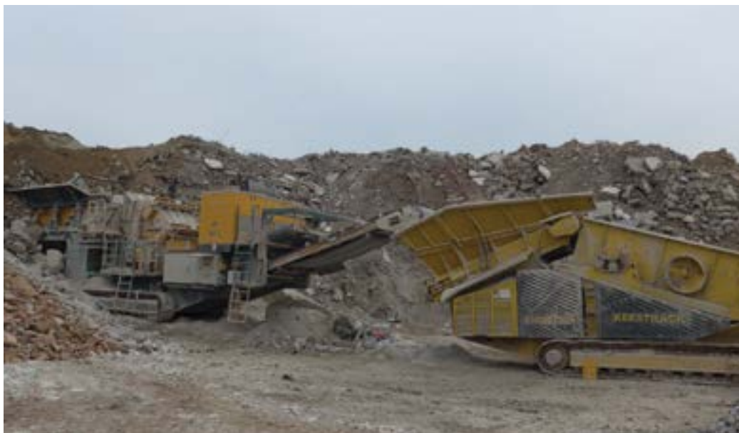
Figure 67: Mobile plant for the processing of mineral construction and demolition waste
