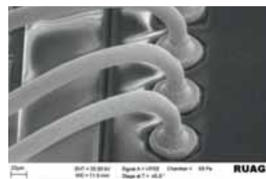
Electron microscope image of bonding detail.
