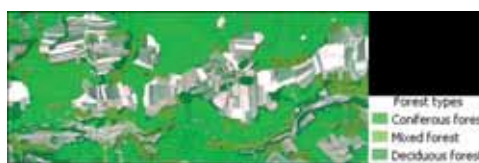
Automatically generated SAR-X Environ forest species map layer for "Bucklige Welt", Lower Austria.
