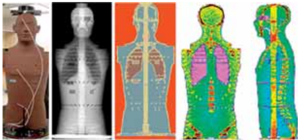
Figure 1: From left to right: The MATROSHKA phantom, a computer tomography of MATROSHKA, the phantom's geometry, simulation results of energy imparted in the phantom due to isotropic photons (front and side view).
