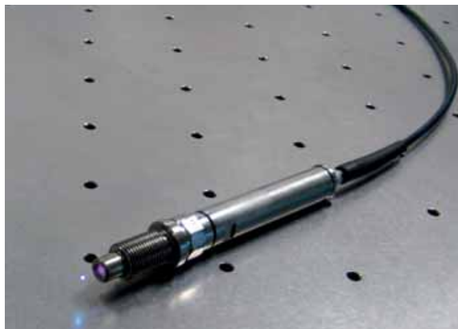
Laser spark plug developed at the Photonics Institute
