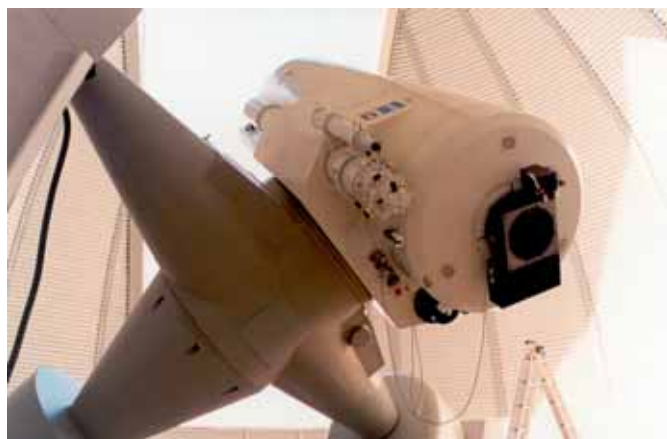
Here the receiver telescope used in this ASAP project is shown, located on the Canary Island of Tenerife.
