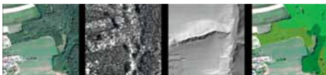
Aerial imagery (left), TerraSAR-X Spotlight data (second left), Digital surface model (second right) and automatically generated SAR-X Environ forest species map layer (right).
