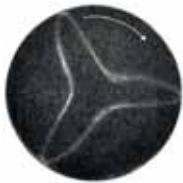
Axial view of a particle accumulation structure with period m=3 in an experiment of Schwabe et al. (2007) (mirror image).
