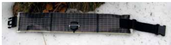
Telemetry test collar with solar panel and GPS antenna
