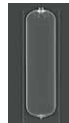
X-ray tomographic picture of a composite tank.
