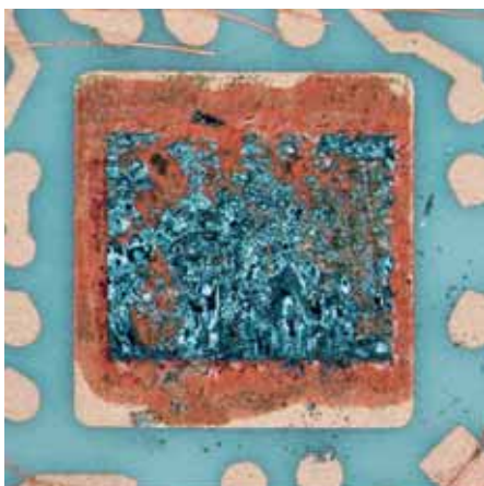
View after destructive die-shear analysis.
