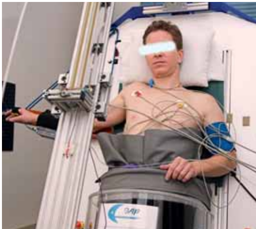
The Insitute's Automated Multi-Stimulation Test Device for freely adjustable, automated, combined change of pitch (+70° head-up to -70° head-down tilt) and yaw (+30° to -30° sideways slant). An additional lower body pressure system allows for POSUP experiment runs.
