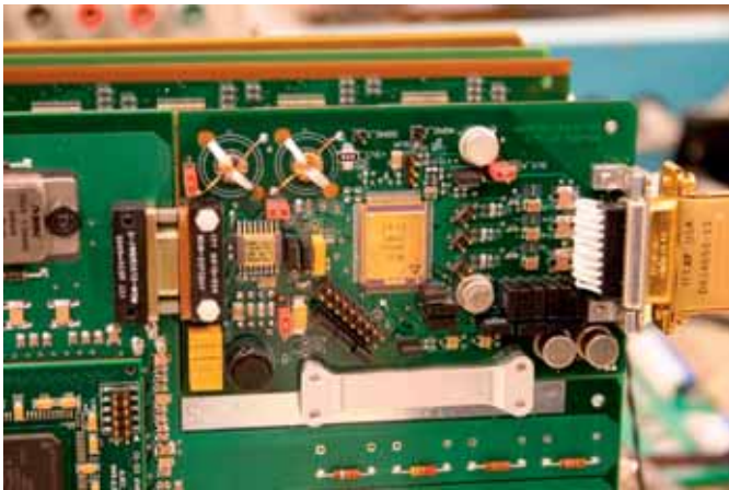
Engineering model of DFG electronics with space qualified Magnetometer Front-end ASIC in the middle (golden lid).
