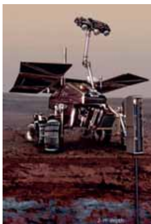
ExoMars rover with drilling device (photo credit ESA)
