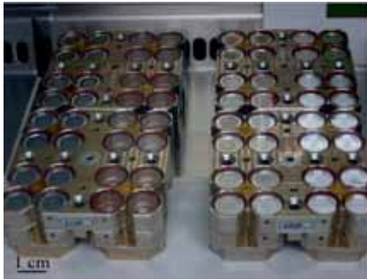
Sample holders of the ISS experiments ADAPT (left) and PROTECT (right) following dismantling in a work bench. Crystals of halite on quartz discs attached with red glue are visible in the left tray.
